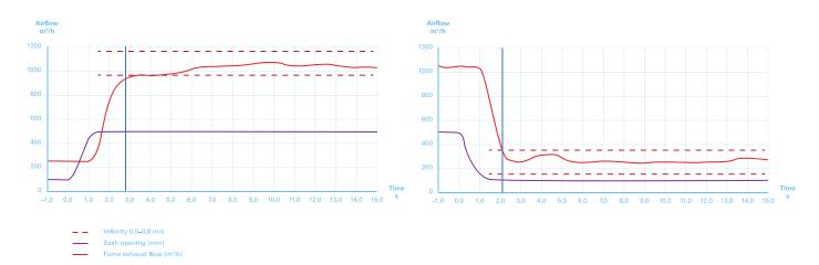
A sash sensor with a very quick reaction time ensures that the airflow is adjusted in less than one second (< 1 s) and the system is stabilised in less than three seconds (< 3 s). When the sash sensor has reached the desired level, the face velocity sensor takes over the control in order to maintain the velocity, taking also into account any blockage caused by people or equipment by the sash opening.
